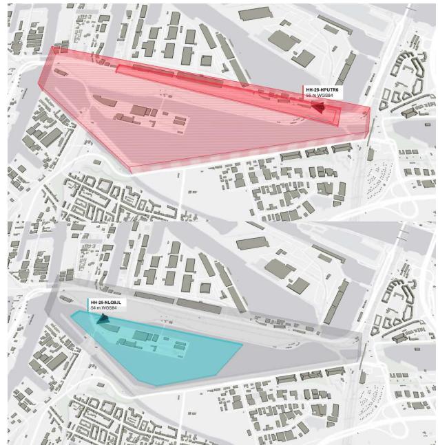
Figure 4. Up: flight with normal status in conflict with TAR (red volume); Down: flight emergency status not in conflict with the same TAR (blue volume).
