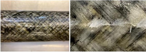
Figure 5: Damaged 63.5 mm pipe after static pressure testing at 85 °C and 6 bar external pressure
