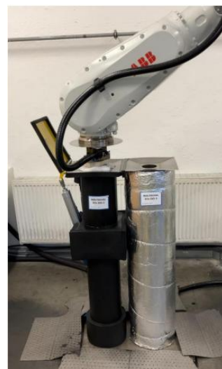
Figure 3: Testing setup for temperature resistance measurements
