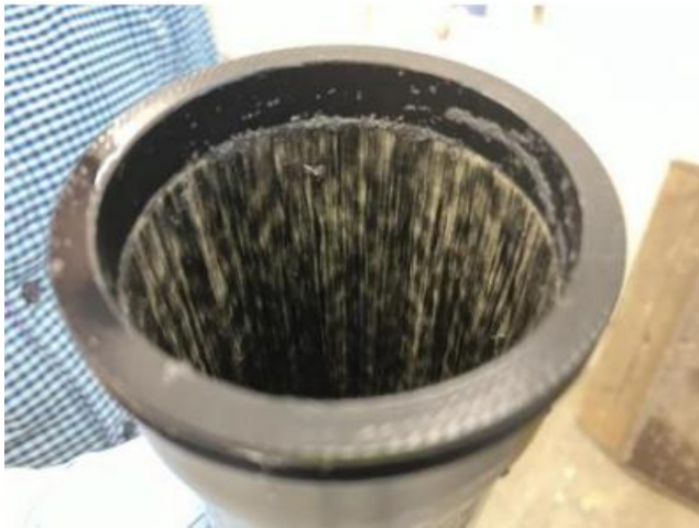
Figure 8: Pipe and end cap with damaged adhesive residues after chemical resistance testing
