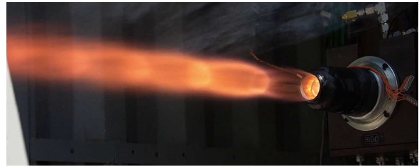
FIG 21. 2000N CFRP engine hotfire test
