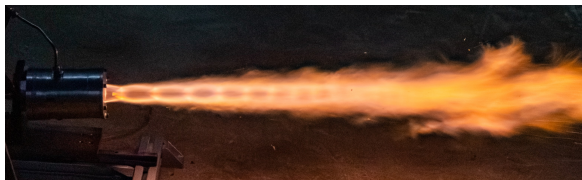
FIG 13. like-like-unlike impingement injector test
