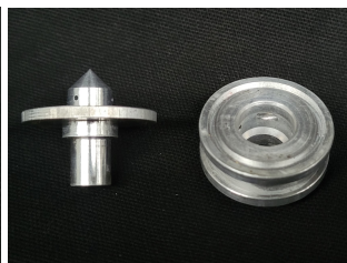
FIG 3. coaxial swirl injector assembly
