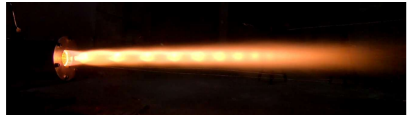
FIG 10. ignition sequence: Ethanol valve open at t = 0.2 s
