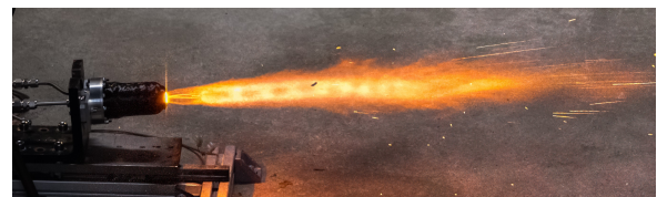
FIG 15. 200N CFRP engine hotfire test
