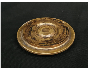
FIG 2. Like-Like-Unlike triplet injector
