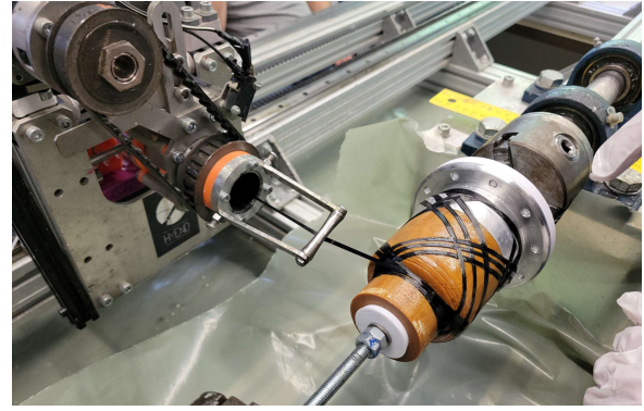
FIG 5. Wet filament winding of the 1000 N CFRP engine pressure casing.
