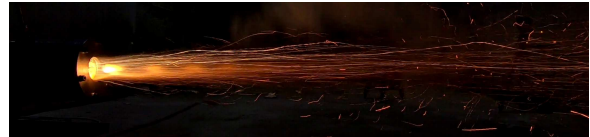
FIG 9. ignition sequence: N_2O valve open at t = 0 s
