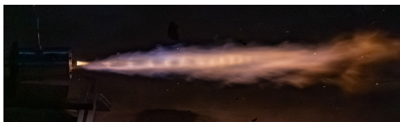
FIG 14. like-like-unlike impingement injector test
