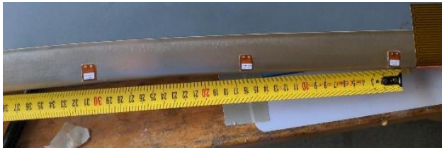
Figure 12 Piezoelectric transducers added to rotor blade leading edge
