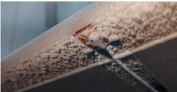
Figure 26 Ice accretion on LILD transducer and test surface
