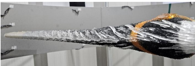
Figure 20 Test case Ice-5 : ice shape at the root of the de-icing blade
