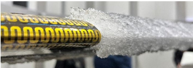
Figure 25 Test case De-Ice-2 : ice shape after de-icing
