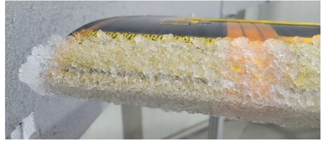
Figure 21 Test case Ice-5 : ice shape at the tip of de-icing blade
