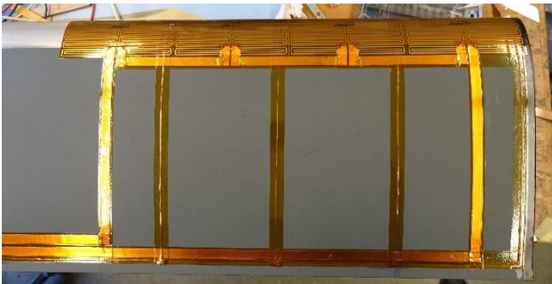
Figure 7 Anti-icing blade heater foils
