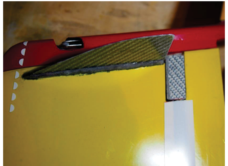
Figure 16, "Frieze Nase" at the aileron, figure shows lower side of the wing
