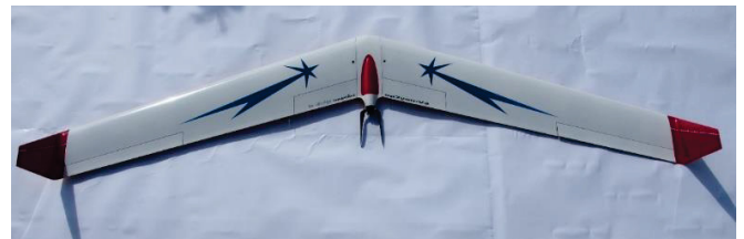
Figure 5, 2m tailless wing drone from [2] as basis for i-con 2 project
