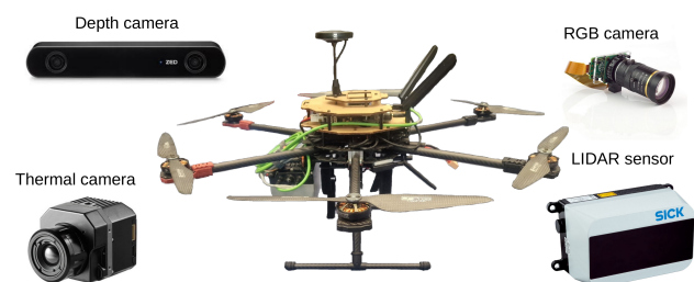
FIG 1. The physical multi-sensor UAS platform used in our flight tests. The integration of advanced sensors into such a compact, low-cost airframe highlights the central challenge addressed by this work: the need for a sophisticated cognitive architecture to transform raw data into intelligent, autonomous actions.
