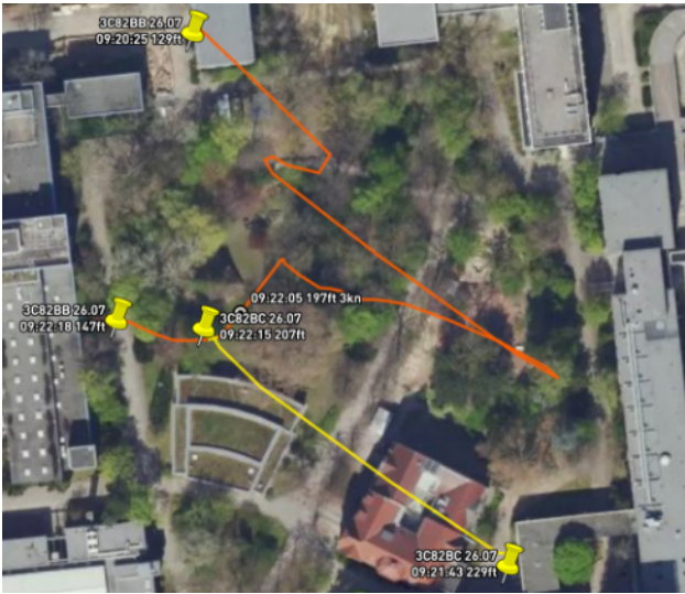
FIG 8. Recordings of the fixed-infrastructure ADS-B system for Drone 7 (orange) and Drone 8 (yellow), showing a pronounced drift for Drone 7 and only a 30 s recording interval for Drone 8.
