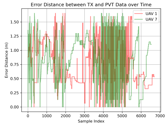
FIG 10. Temporal evolution of the positional error between the transmitted ADS-L position and the recorded ground truth for Drone 1 and Drone 7.
