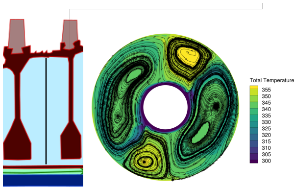
FIG 6. Temperature distribution in the cavity mid plane with the location indicated by line
