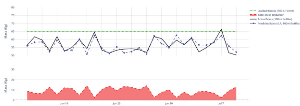
FIG 5. Loaded water bottle mass, predicted mass and mass reduction (FRA-DEL).
