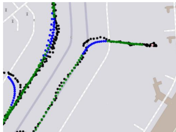
Figure 3: Comparison of raw data (black points) and Hatch filter applied (green and blue points).
