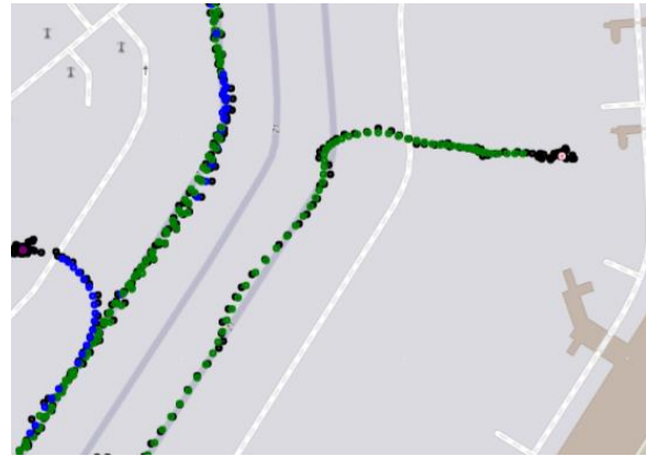
Figure 2: Comparison of raw data (black points) and Gaussian filter applied (green and blue points).
