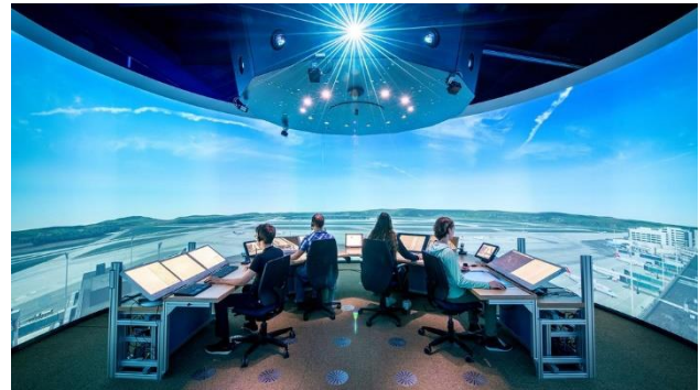
Figure 1: The ATS360 tower simulator at the DLR Braunschweig.
