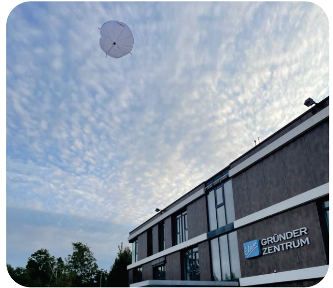
Image 8 Wind-influenced load test w. tethered system
