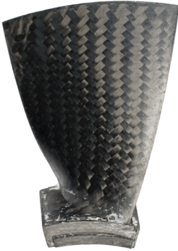
FIG 3. CFRP blades manufactured at the institute Ref. [7]
