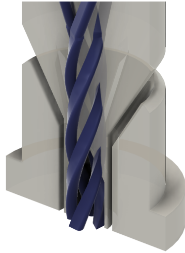
FIG 8. Swirl injector internal oxidizer flow.
