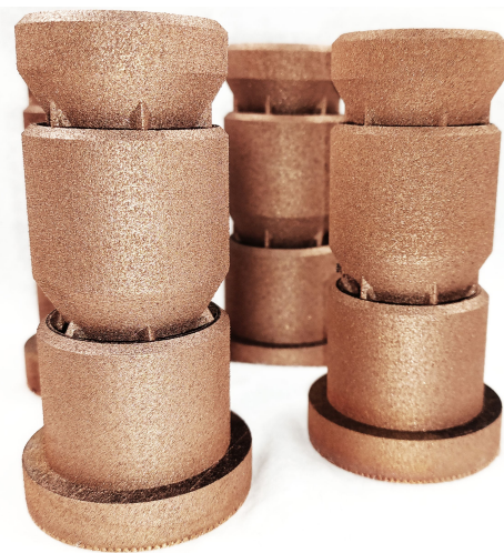
FIG 9. Additively manufactured injectors, before post-processing.
