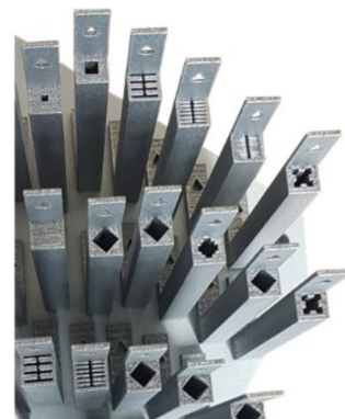
FIG 22. Hollow conductors with various inner profile shapes serve as cavities for phase change materials buffering temperature peaks by absorbing thermal power [71].
