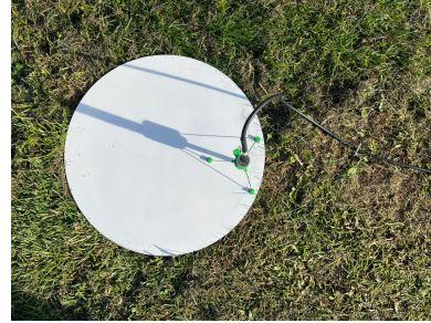
FIG 3. Microphone placed on ground plate.
