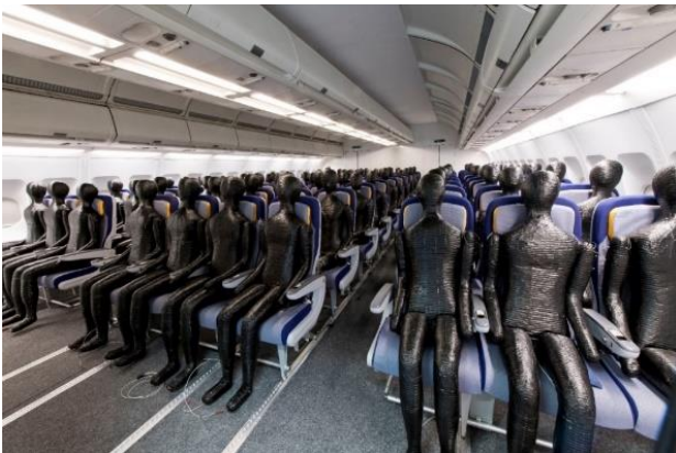
FIG 1. Interior of the cabin mock-up with thermal manikins.
