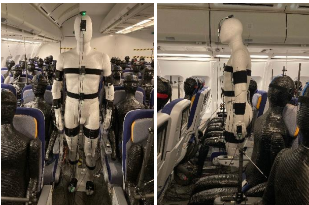
FIG 4. Manikin with 16 Equites comfort probes.
