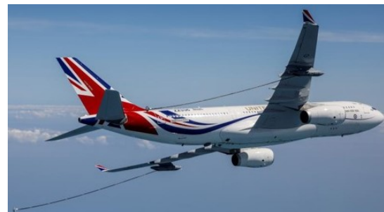
FIG 2. Example of a tanker equipped for probe-drogue-refuelling [5]
