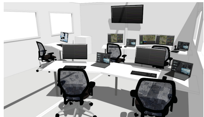
FIG 6. Concept of the Ground Segment Operations (GS-Ops). The remote pilot and support station are located on the front right hand side of the operations center. The flight director and flight test engineer are placed behind. On the left hand side the payload operator station is positioned.
