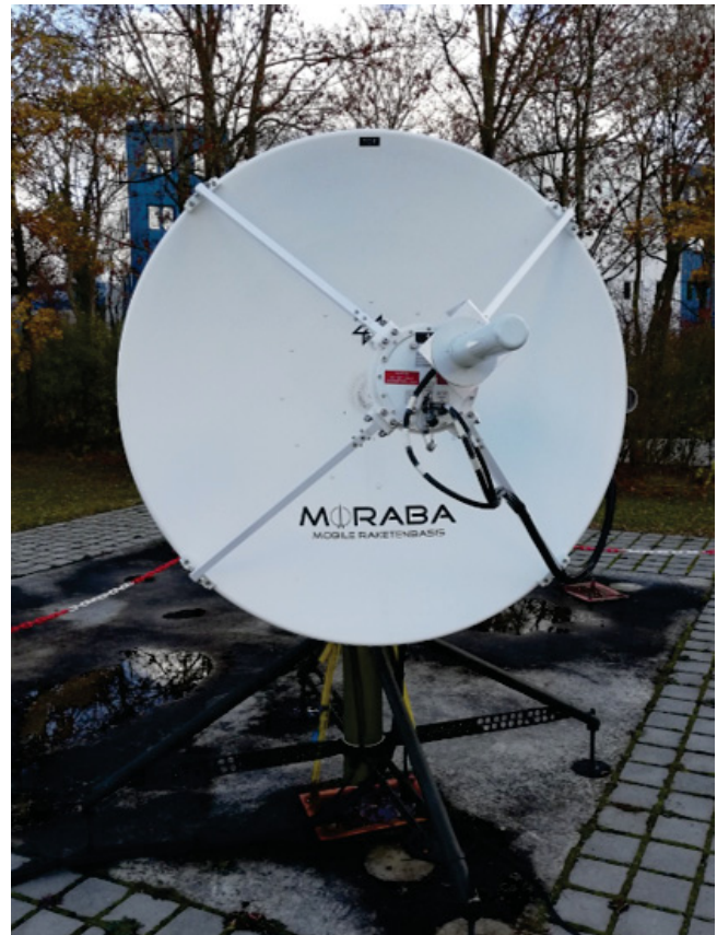
FIG 4. Exemplary combined X- and S-band parabolic antenna with a dish-size of 1.5m diameter. This antenna is owned by DLR and was used for first communication tests on ground.
