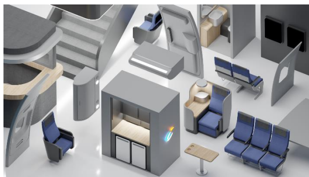
Figure 6: An excerpt of the collection of the existing predefined cabin objects in the custom BHL model database.
