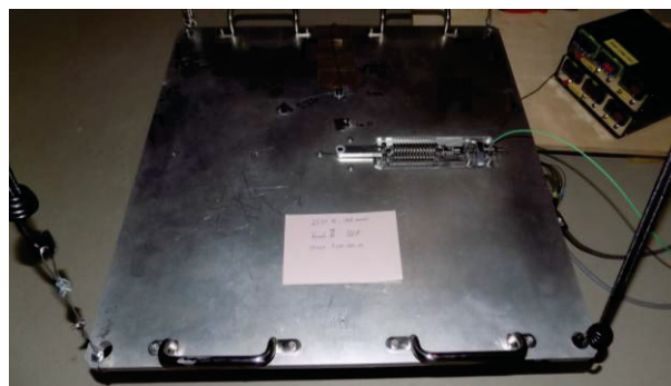
FIGURE 7. Example Test setup for shock measurement
