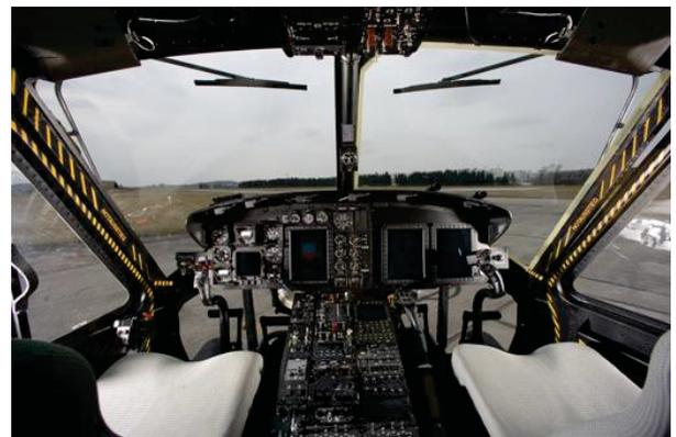
Figure 6 MAT cockpit with safety pilot environment (left side) and experimental pilot environment (right sight)
