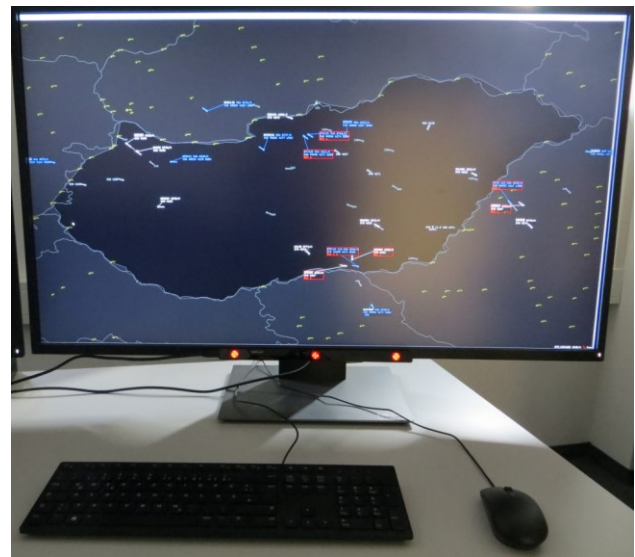
FIGURE 2. Sectorless Controller Working Position Prototype in the “Complete Airspace” Design
