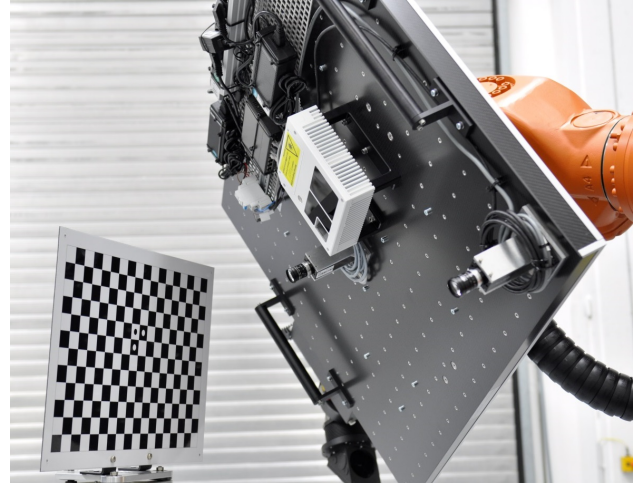
FIGURE 4. Carbon fiber optical breadboard on robot 1. For flexible mounting of sensors and associated equipment. CCD camera calibration pattern in front of the breadboard.
