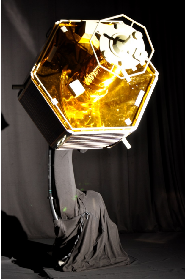
FIGURE 3. True-to-scale target mockup with real MLI and solar arrays mounted on robot 2. Black curtain in background and around robot to mimic dark space background.
