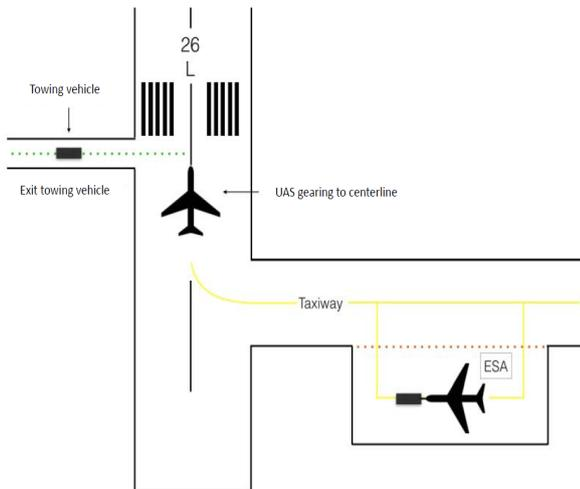
FIGURE 3. Aerodrome concept line-up with “Engine-Start-Area” (ESA) for RPA [9]
