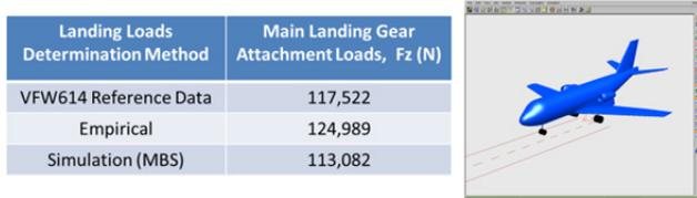
**Figure 11:** An MBS model of VFW 614 for the 3 Wheel-Landing case and the comparison of main landing gear attachment loads result from the empirical method and from the MBS
