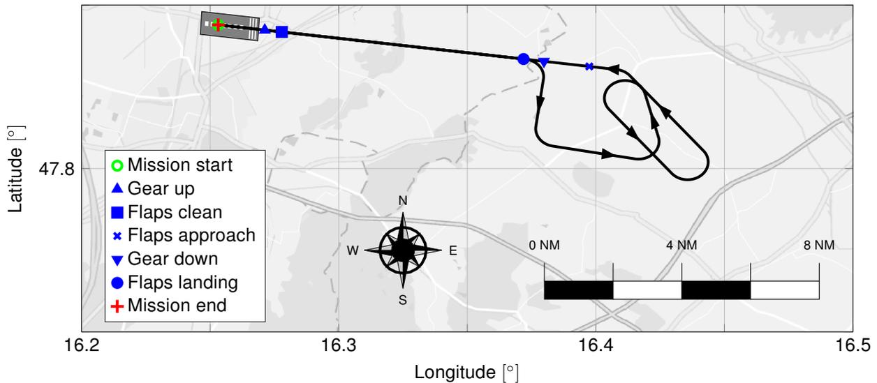
Figure 3: Automatic Landing Mission - Reference Ground Track.
