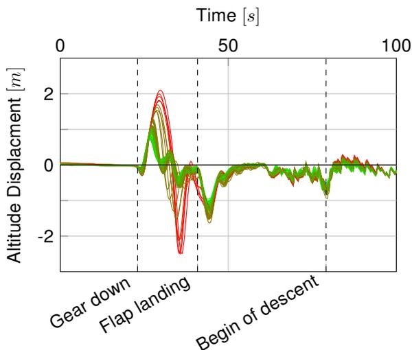
Figure 7: Monte Carlo Study, Aerodyn. Parameters  $\pm 70\%$ .
