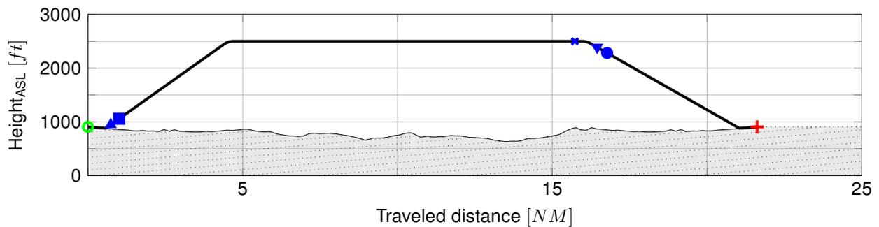
Figure 4: Automatic Landing Mission - Reference Altitude.
