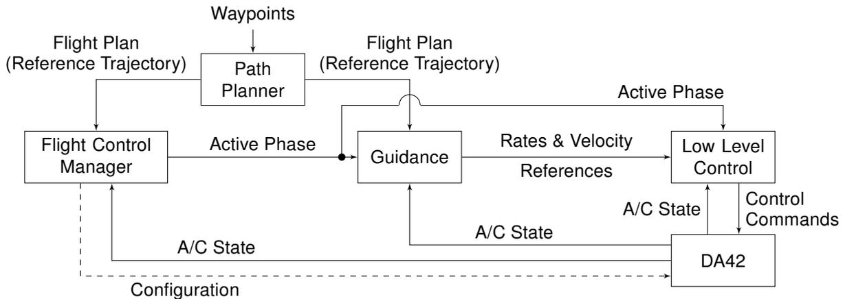
Figure 2: Flight Control Laws Structure.
