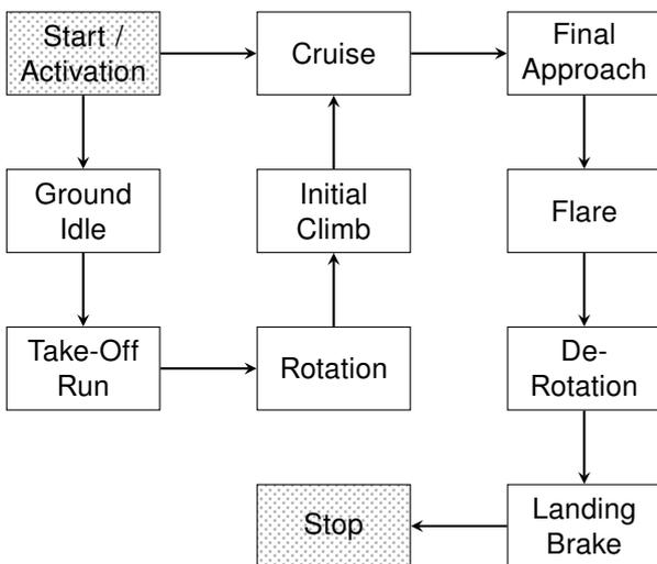
Figure 5: Flight Control Manager State Machine.
