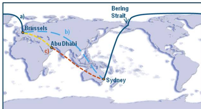
Figure 1: The three considered trajectories from Brussels to Sydney: a) hypersonic overflight of Bering Strait (solid), b) first portion of flight trajectory in eastern direction to Volgograd subsonic cruise, followed by hypersonic cruise to Sydney (dashed), and for reference c) subsonic cruise (dotted), with gas stop in Abu Dhabi.
