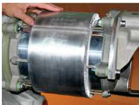
Figure 10: Tesla Electric Roadster Sport electric motor, peak power 225 kW, 32 kg, here shown with mounted flanges [15]
