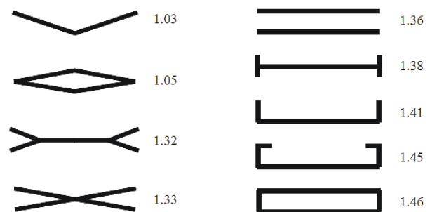
FIG 1. Highly non-planar lifting systems, Kroo [17]
