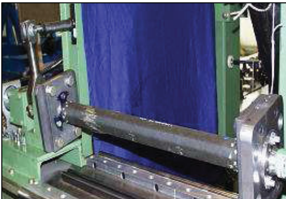
Fig. 19 EC135 carbon composite tail rotor drive shaft on test set-up
