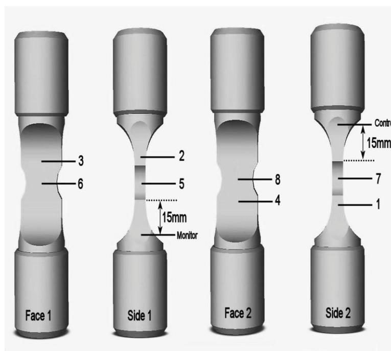
**Figure 5:** Stage 1 thermal profiling showing thermocouple positions. A total of 10 TC's are spot welded to the specimen surface at positions around the specimen, and control and monitor TC's at the adjacent shoulders.
