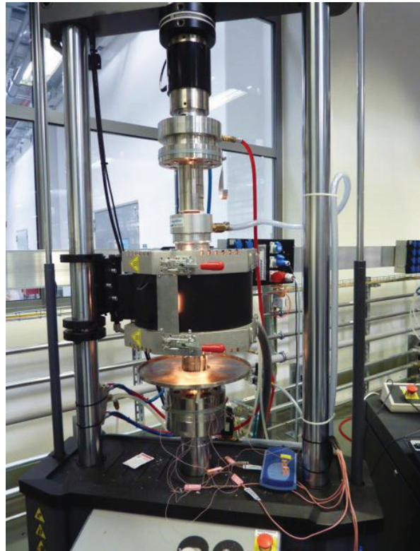
**Figure 1:** The stress controlled TMF testing system consists of a MTS 250kN *Landmark* load frame, 12kW Infra-red radiant lamp furnace, and facility compressed air cooling additionally accelerated with an *Exair* air amplifier, all controlled by the MTS *TestSuite* software.
