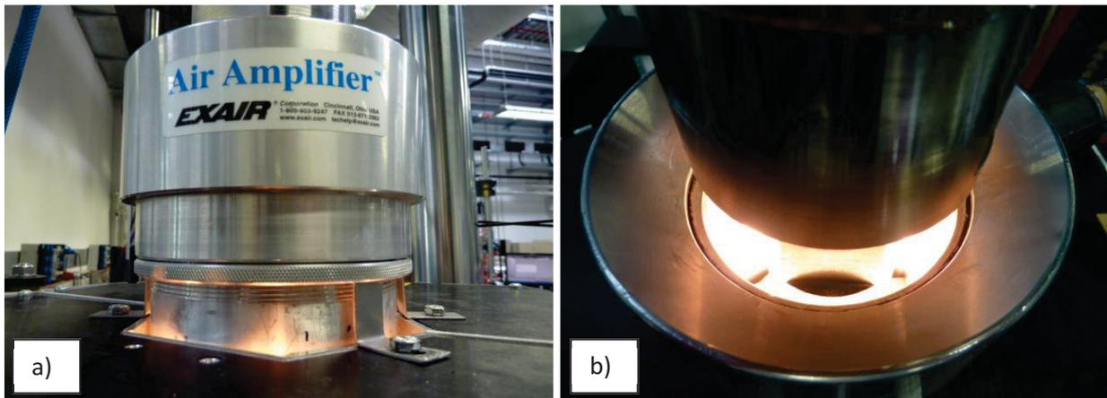
**Figure 4:** The Exair air amplifier, situated at the top of the furnace. a) Centred at the top of the furnace it accelerates MTOC facility compressed air up to  $35.4\text{m}^3$  per minute (1250 SCFM) at 517 kPa (75psi). b) View looking into the top of the furnace at over  $400^\circ\text{C}$ .
