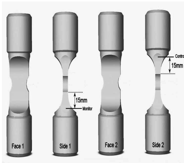
**Figure 7:** Stage 3 thermal profiling. Only the control and monitor thermocouples remain on the specimen shoulders
