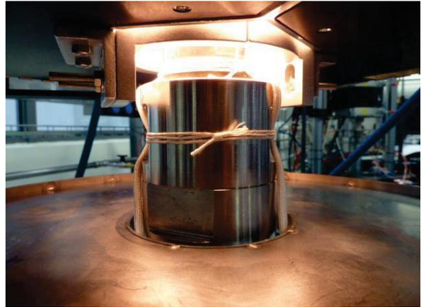
**Figure 3:** The base of the furnace where the hot air is exhausted. The disc under the furnace dissipates the heat away from the machine. It additionally acts as protection should a part of a hot specimen fall out of the furnace. Centralising brackets are located underneath to ensure accurate positioning of the furnace once it is closed.
