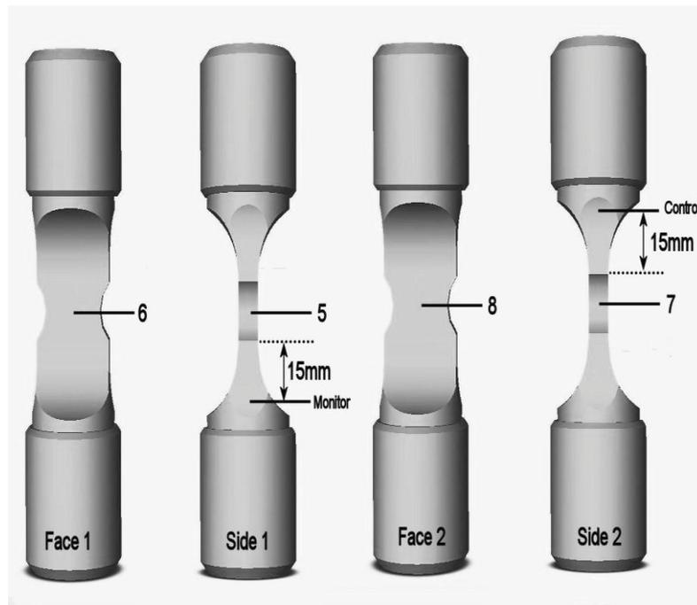
**Figure 6:** Stage 2 thermal profiling. 4 TC's are positioned around the gauge section of the specimen and control and monitor TC's at the adjacent shoulders.
