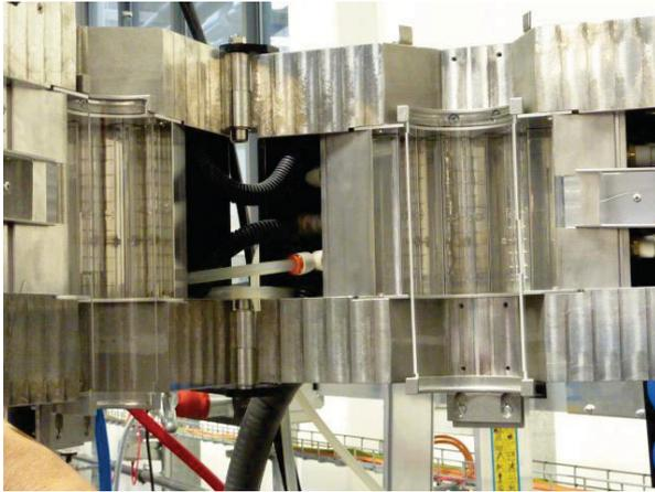
**Figure 2:** Internal view of the Infra-red 12kW Radiant lamp furnace. 12 vertically mounted lamps provide the rapid heating rates required for this type of test. The quartz glass liners enable the cooling air to pass smoothly through the furnace.
