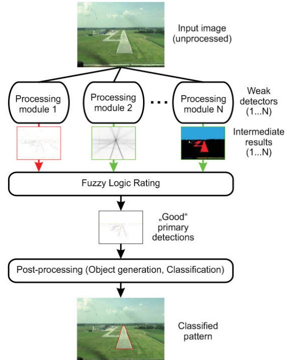
Fig. 2: Task parallelisation (N parallel processing modules)
