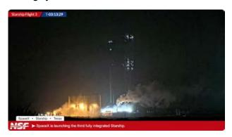
14 March 2024 at 13:25 UTC, SpaceX launches the third integrated flight test IFT-3 from the company's Starbase launch facility in Boca China, Texas. A complement of 33 Raptor engines, fuelled by super-cooled liquid methane and liquid hydrogen powered the Super Heavy booster with Starship stacked on top.
