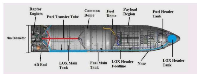
Diagram of Starship's internal structure. Not shown in this diagram are the flaps: the aft flaps are placed at the bottom (or left in this orientation), and the forward flaps are placed at the top (here, right) portion of the spaceship.
