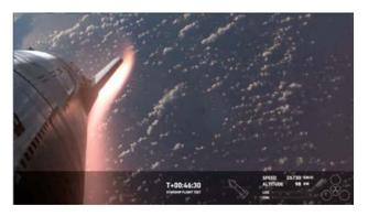
SpaceX's Flight 3 upper stage glows orange as it heats up during re-entry during test flight 3 on March 14, 2024. (Image credit: SpaceX) Telemetry data continued streaming from Starship back to SpaceX mission control until it reached an altitude of around 65 km. Then, the team lost two key pieces of communication at the same time:
