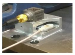
Sensors are packaged into a light weight assembly with a small footprint
