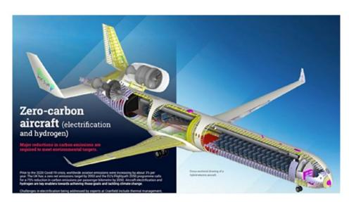
Figure 1: Cranfield concept design for a future hybrid hydrogen-electric commuter aircraft. (© Cranfield University)
