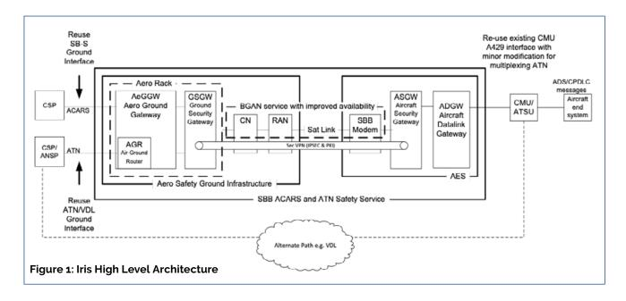
The main **Iris ground segment** components are integrated in the Aero Rack:
