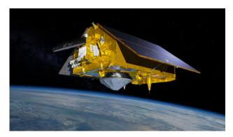
Illustration of the Sentinel-6 Michael Freilich spacecraft in orbit above Earth with its deployable solar panels extended
