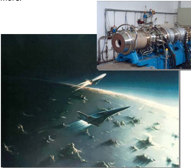
Content of the german national hypersonic research program was once more a two stage to orbit space plane, this time with a combined turbo-ram jet propulsion.
