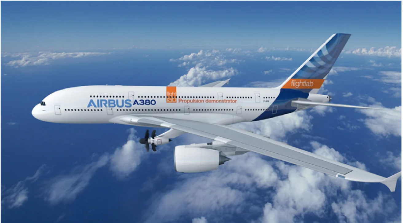
Figure 2 : The A380 super jumbo is the flight test demonstrator for the development of advanced propulsion technologies, among which the Open Fan. © Airbus.
