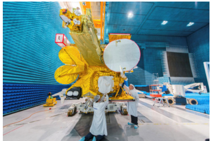
Fig. 2: Eutelsat 9B Satellite with EDRS-A Payload (LCT on Top-Floor with a white cover for protection) at Airbus
