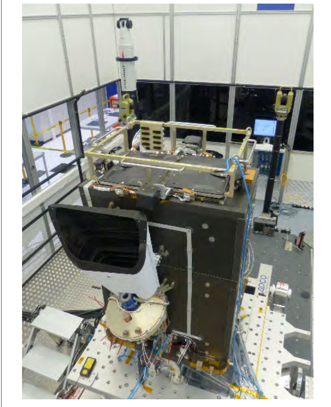
Fig.7b: Up: Aperture Cover Qualification Models Bottom: Calibration assembly and ACV QM assembled on the Instrument EM
