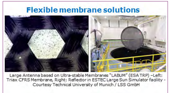
Figure 6: Flexible membrane made of CFRS as RF reflective surface
