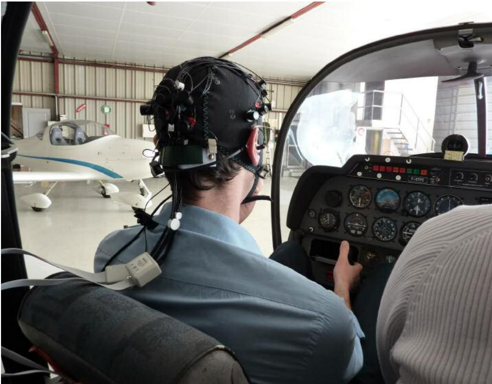
Illustration 6: Toulouse-based researchers are monitoring a pilot's brain activity in flight, equipping his head for functional near infrared spectroscopy.
