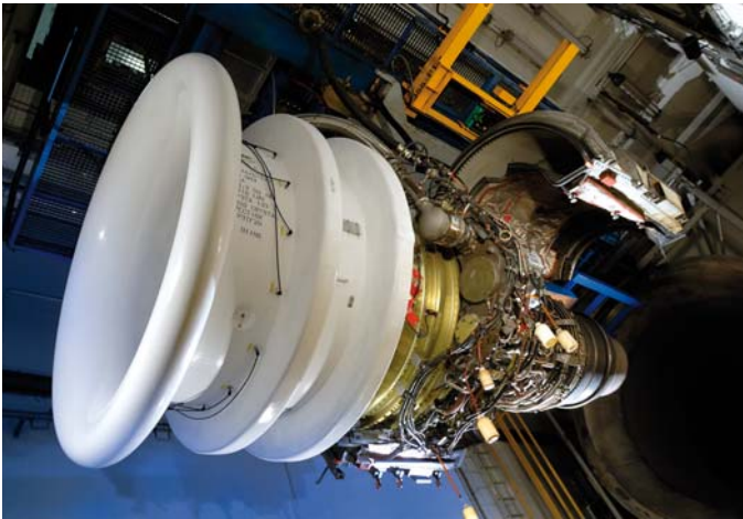
Figure 2. CFM Programme initiated in early 2007 on a CFM56-7 engine: the first test run at Snecma using a first generation alternative fuel.
