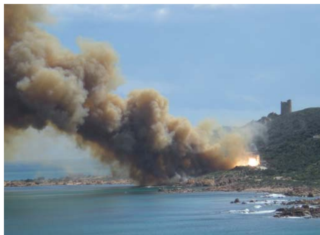
Figure 1. : On 28 April 2009, the final qualification test firing of the third stage solid propellant motor of VEGA took place at the Salto di Quirra Interforce Test Range in Sardinia, Italy. (Credit ESA)
