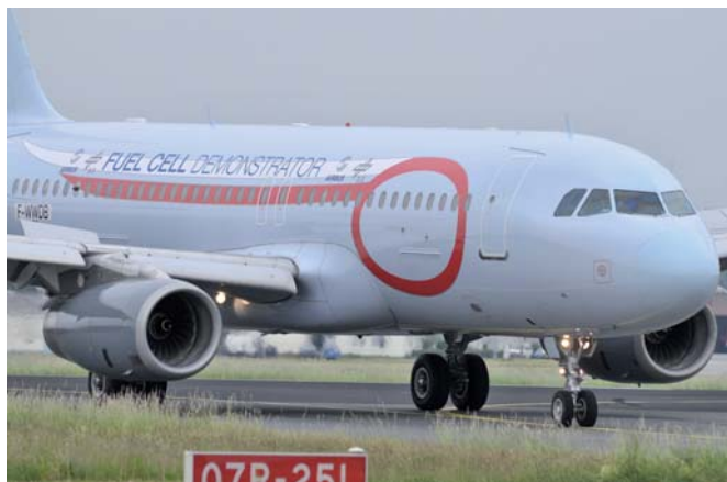
3. ILA 2008. Passenger & Transport Aircraft. The DLR Airbus A320-232 ATRA contains a Fuel Cell System from Michelin. This is a common project of Airbus and the DLR.
